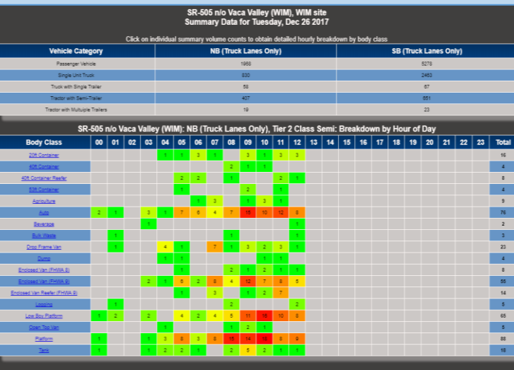
Sample Data Summary Visualization Source: University of California, Institute of Transportation Studies, "Truck Activity Monitoring System (TAMS)". Available at: http://freight.its.uci.edu/tams/
